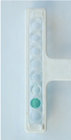
Negative test – i.e. Wells 1 to 5 show no colour change. Only Well 7 (Positive Control) is positive.
